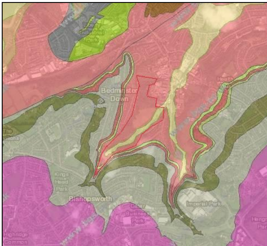
Geological map covering Manor Woods Valley (centre) Pink layer = Mercia Mudstone Group, Yellow layer = overlying fluvial deposits
